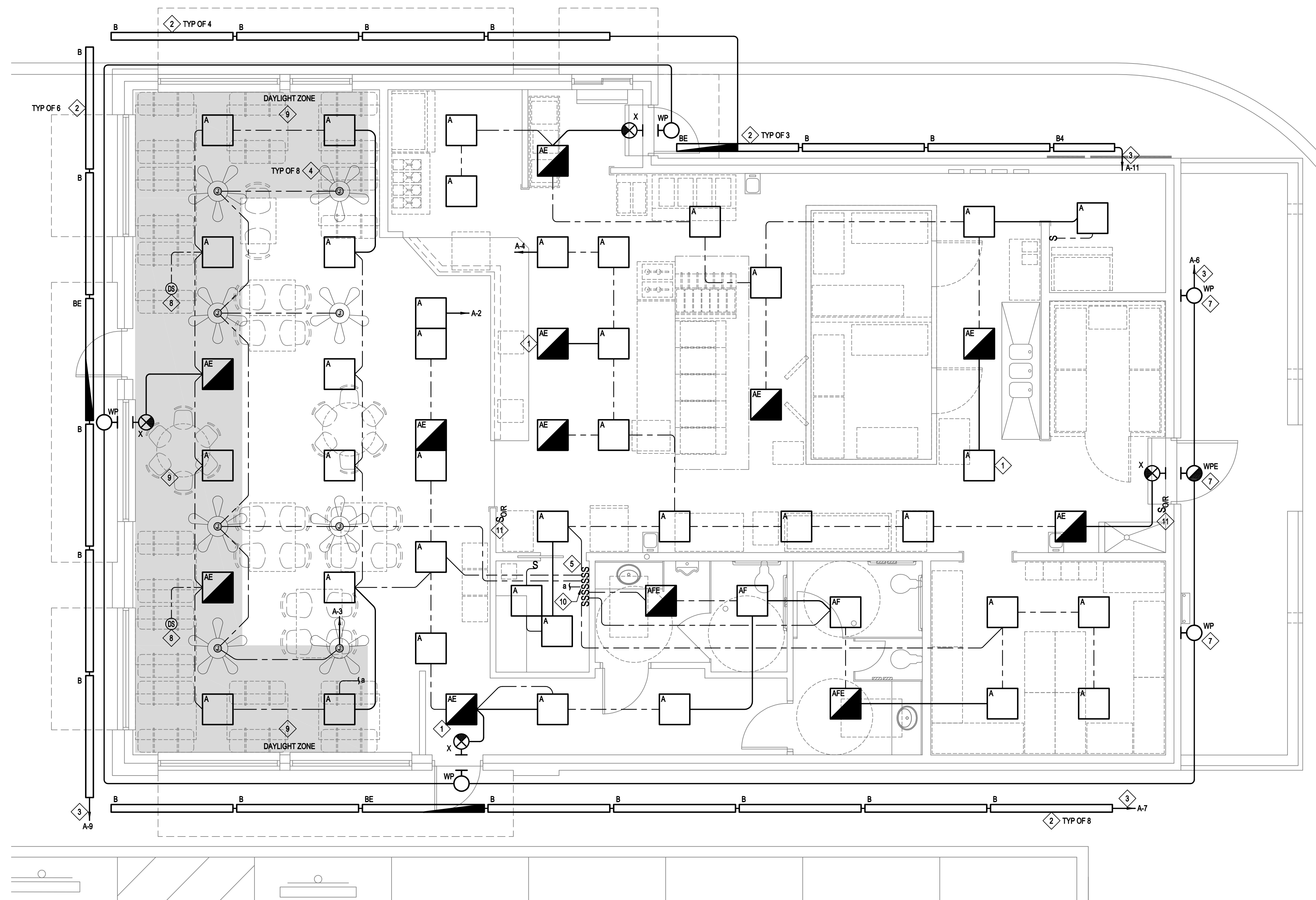
1 ELECTRICAL FLOOR PLAN - LIGHTING SCALE: 1/4" = 1'-0"
